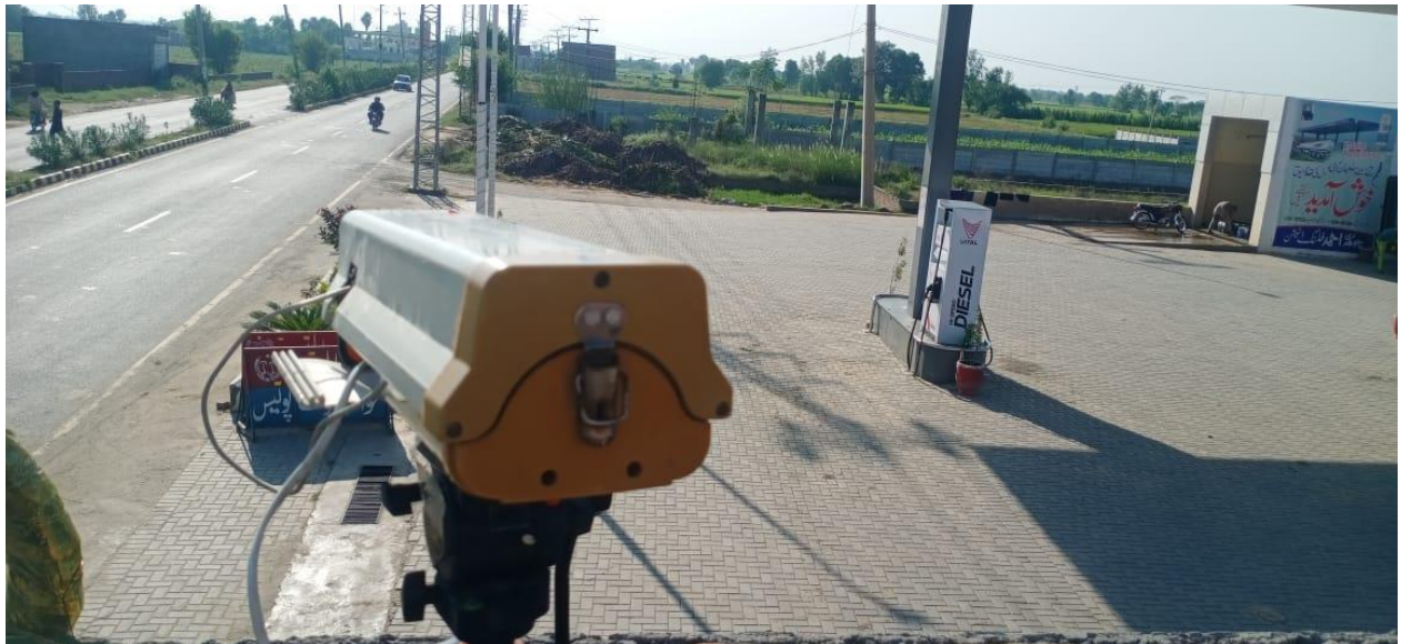
Figure 2 - Vehicle Counting Device Mounted at Traffic Survey Site
