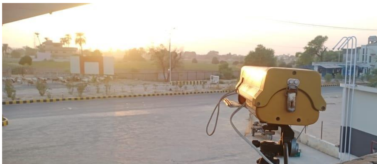
Figure 2 - Vehicle Counting Device Mounted at Traffic Survey Site
