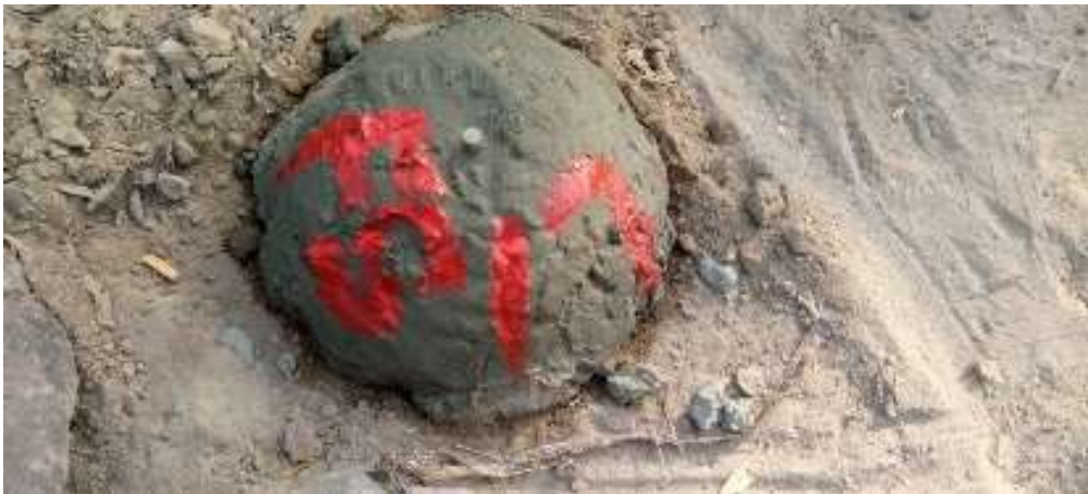
FS 17 CONCRETE MONUMENT WITH STEEL NAIL AT CENTER
