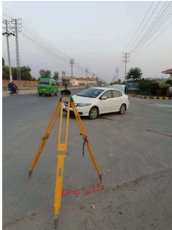
GPS BASE STATION AT POINT FS 25 COLLECTING DATA
