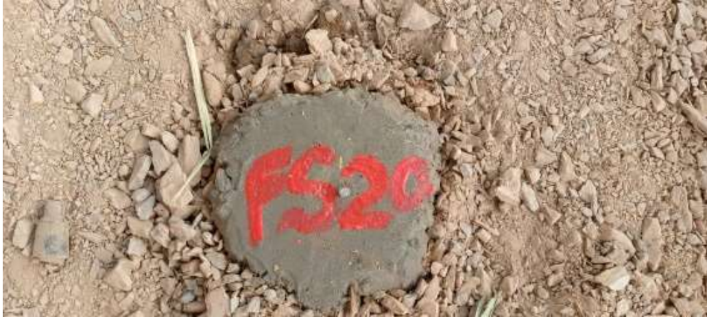
FS 20 CONCRETE MONUMENT WITH STEEL NAIL AT CENTER
