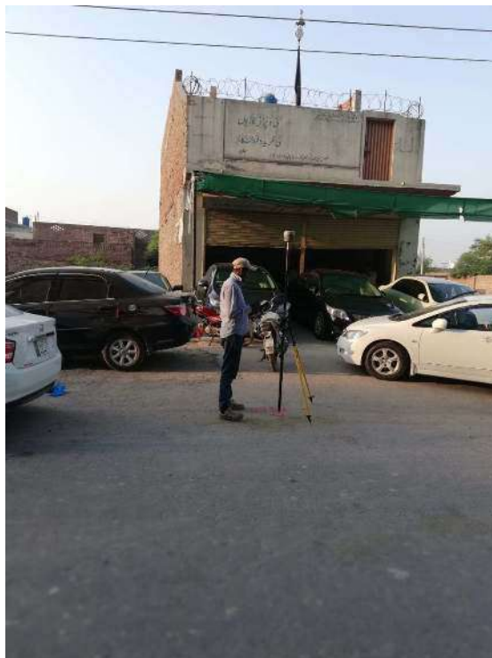
STATIC POINT OBSERVATION ALONG THE ROAD
