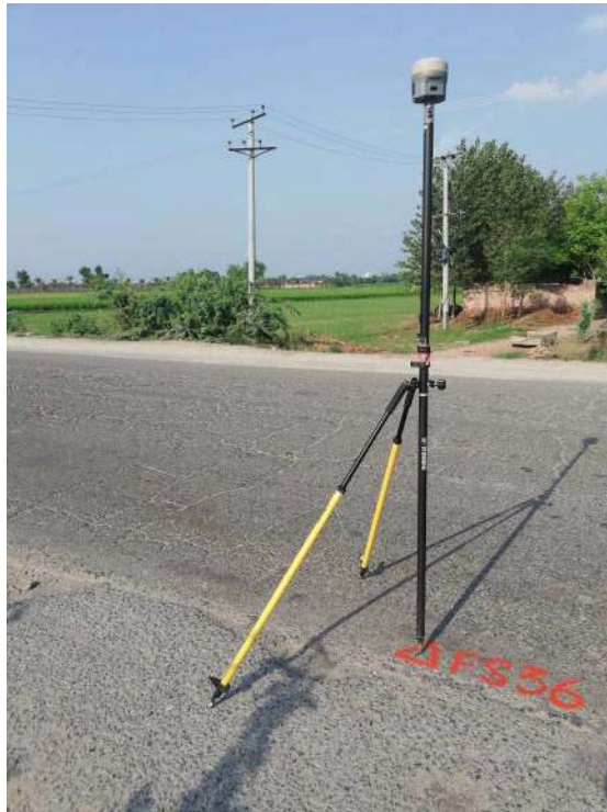
STATIC POINT (FS36) OBSERVATION ALONG THE ROAD
