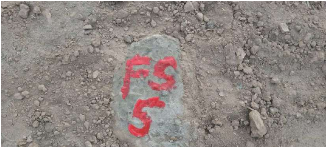
FS 5 CONCRETE MONUMENT WITH STEEL NAIL AT CENTER
