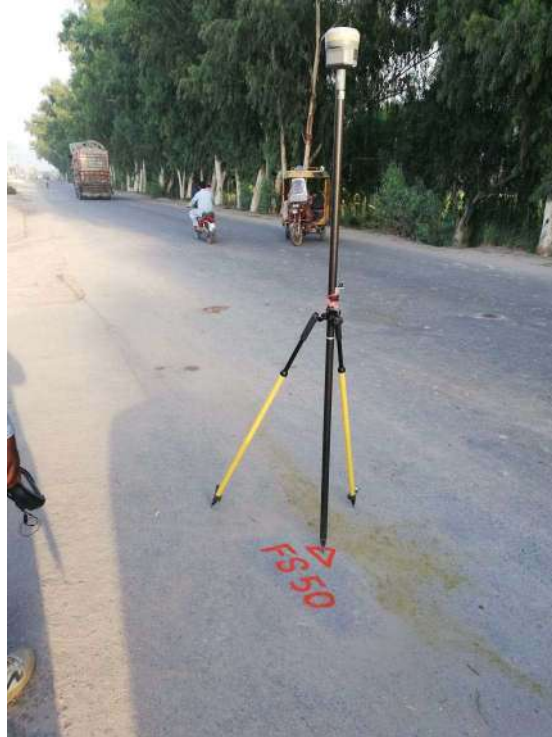
STATIC POINT (FS50) OBSERVATION ALONG THE ROAD
