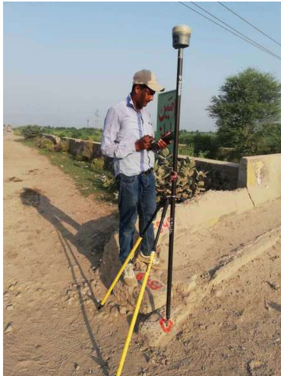
STATIC POINT (FS49) OBSERVATION ALONG THE ROAD AT BRIDGE
